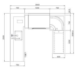
With a length of only 2842 mm, this setup option is ideal for kitchens with limited space for the washing area. It saves a significant amount of space. Even in the smallest areas, optimum washing capacity can be achieved with the STR 110.
